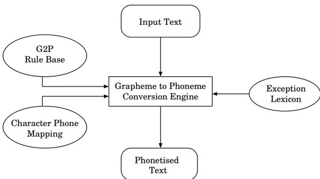
Fig. 1. G2P Converter Architecture
